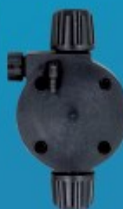
Testa pompa PVC completa con valvola sfera e tenute FPM o EPDM PVC pump head for high flow rate ( 20 lt/h up to 50 lt/h) complete with ball injection valves (ceramic balls) FPM or EPDM seals
